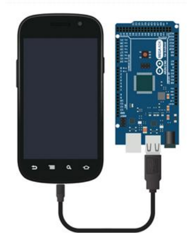
Figure 10: An Arduino-ADK connected to an Android Mobile Phone.
